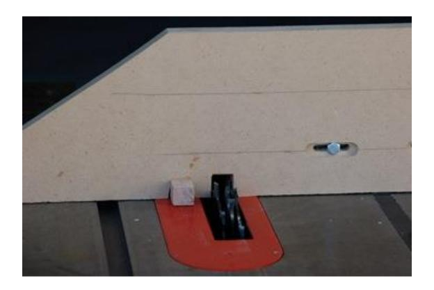
This is a picture of a simple Box Joint jig that I have attached to my Miter Gauge. You can make the joint cuts for a hive body in less than 5 minutes.
